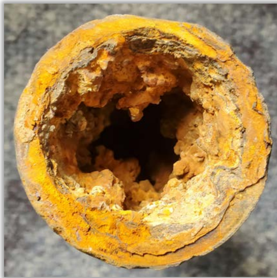
Corroded & Aging Smithville Waterline Segments
